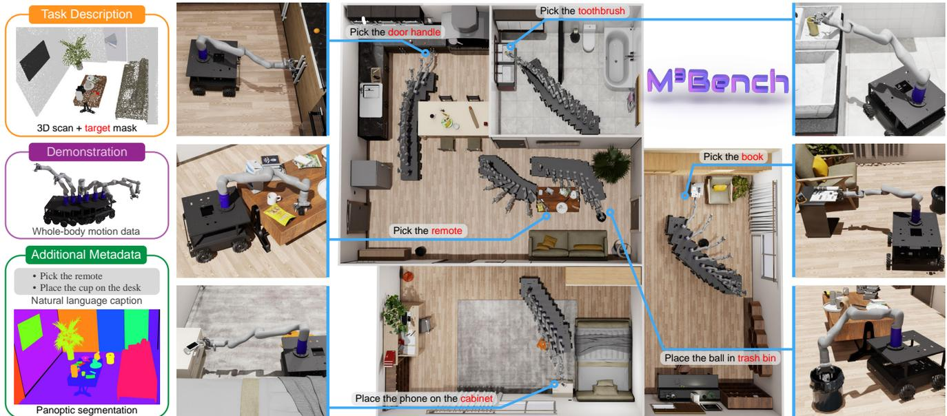
Fig. 1: The M<sup>3</sup>Bench benchmark challenges mobile manipulators to generate whole-body motion trajectories for object manipulation in 3D scenes. Given a 3D scan, a target segmentation mask, and a task description, the robot must understand its embodiment, environment, and task objectives to produce coordinated motions for picking or placing objects.
